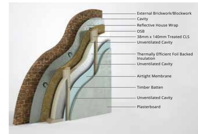
Wall Option 2 U-value - 0.17 W/m 2 k Overall Width - 339mm
